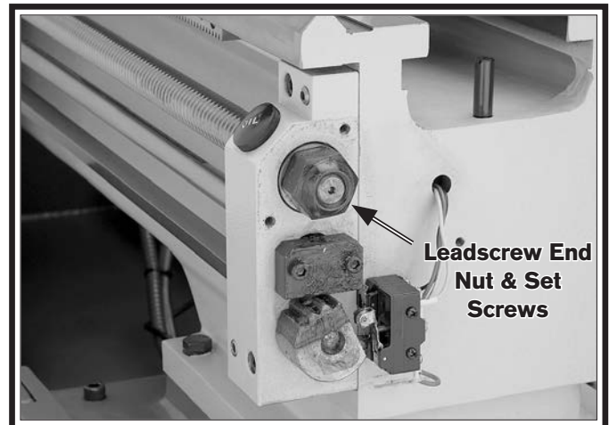
Figure 123. Leadscrew end nut.
